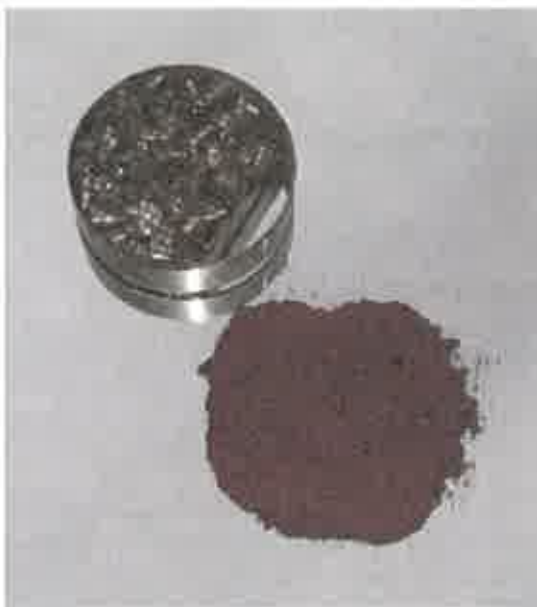
Picture: A quantity of ash (mineral, iron containing ash) which was filtered from the flue gas by the ABCAT modules after the burn of approx. 20 kg air-dry beech. This ash, if not filtered by the ABCAT, would have been emitted into the atmosphere.
